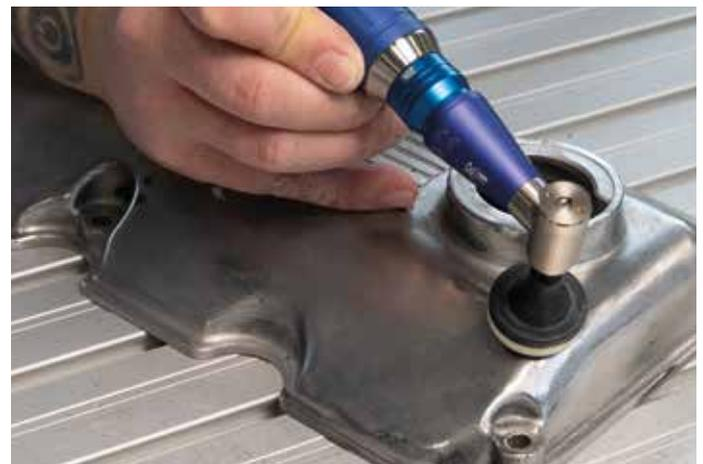
Aluminium polishing with angle-handpiece and felt
